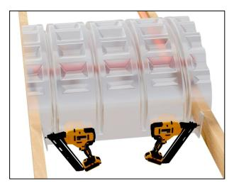
Perpendicular-to-Rafter Installation: Fold the (4) corner mounting tabs outward along the embossed fold lines. Place the Rafter Runner between the joists centered over the pipe/utility. Confirm the first Rafter Runner vertical walls are installed at 22.5" wide. Install 2-3 fasteners in each of the mounting tabs. Place the next Rafter Runner in the adjacent joist space and confirm the 1.5" overlap of the two Runners is maintained. Install the tab fasteners. Repeat as needed.
